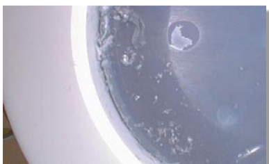
Abrasion of a standard PTFE liner
