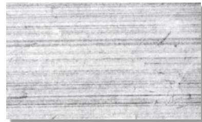
25x enlargement of the surface of a unprepared ULTRAFLO ® liner
