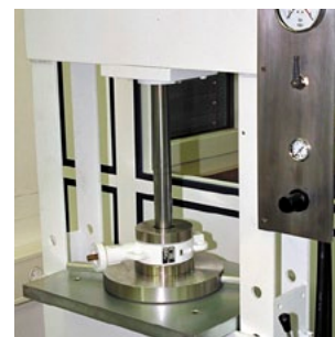
Tightness test with HP nitrogen
