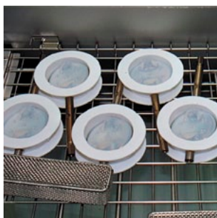
Decontamination by ultrasonic cleaning
